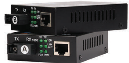
10/100M Single Mode Single Fiber, BiDi, 20km, SC, Tx1310/Rx1550nm & Tx1550/Rx1310nm
