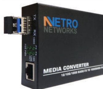
10/100/1000M SFP Media Converter 1G External AC 220V (Without SFP)
